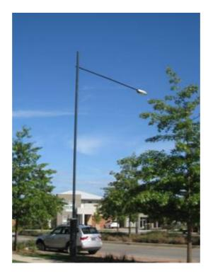
Plate 1 Example of lighting pole type - VicPole and Dulux charcoal colour 32999.
