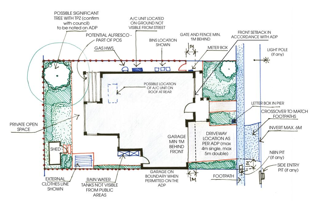
Figure 1: Site plan sketch (typical allotments) - general requirements
