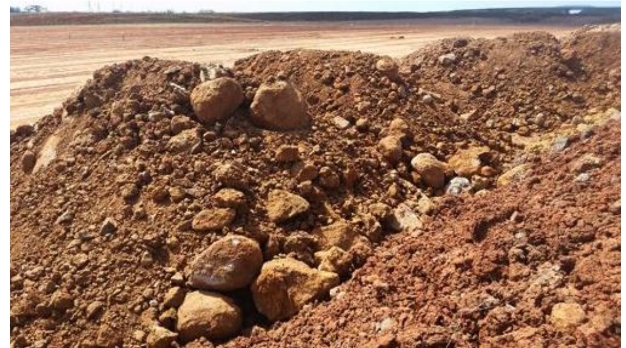
Dry gravelly clay fill with oversize boulders present (imported from Werribee) - E4
