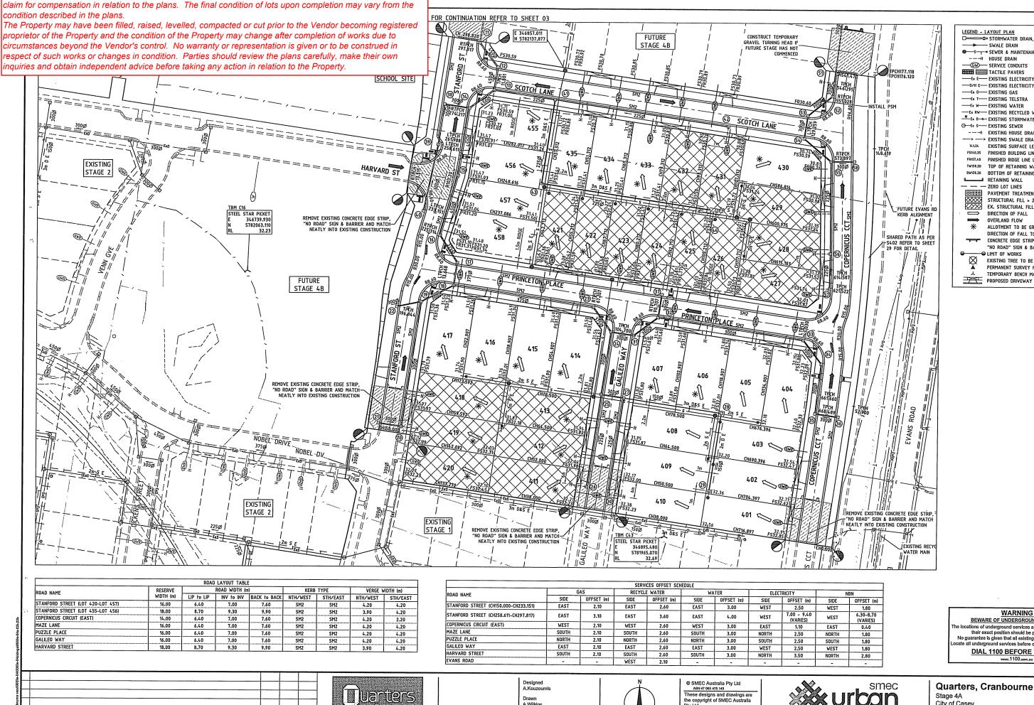
LEGEND - LAYOUT PLAN STORMWATER DRAIN, PIT & PROPERTY INLET - SWALE DRAIN STY SEWER & MAINTENANCE STRUCTURES --- HOUSE DRAIN -GW- SERVICE CONDUITS TACTILE PAVERS ---Ex E---- EXISTING FLECTRICITY (UNDERGROUND) Ex G-EXISTING GAS ----Ex T---- EXISTING TELSTRA Ex W- EXISTING WATER EXISTING RECYCLED WATER
