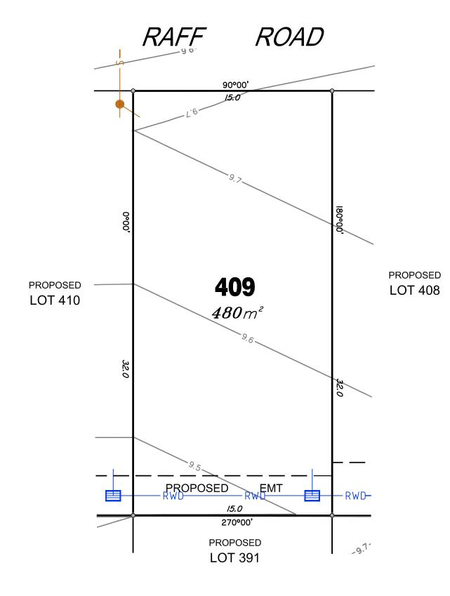
Final surface contours based on A.H.D. datum at an interval of 0.1m, shown as: —— I·0 —
